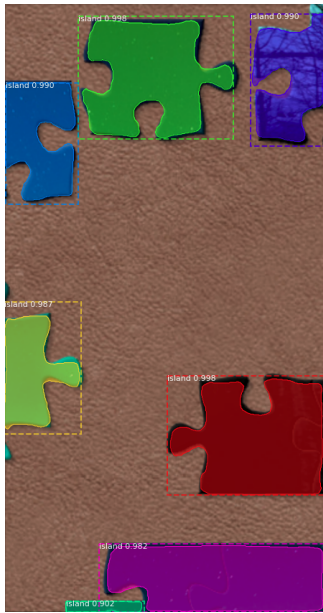
Figure 9: The output from Mask-RCNN border extraction for a image of puzzle pieces that have a textured/fuzzy background. The image shows what the model thinks are island pieces, along with the confidence value for each.
