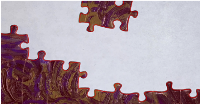
Figure 10: The output from adaptive thresholding border extraction for a image of puzzle pieces under ideal conditions. Here we see the extracted border as a red 'transparent overlay on top of the original image with an opaque border outline.
