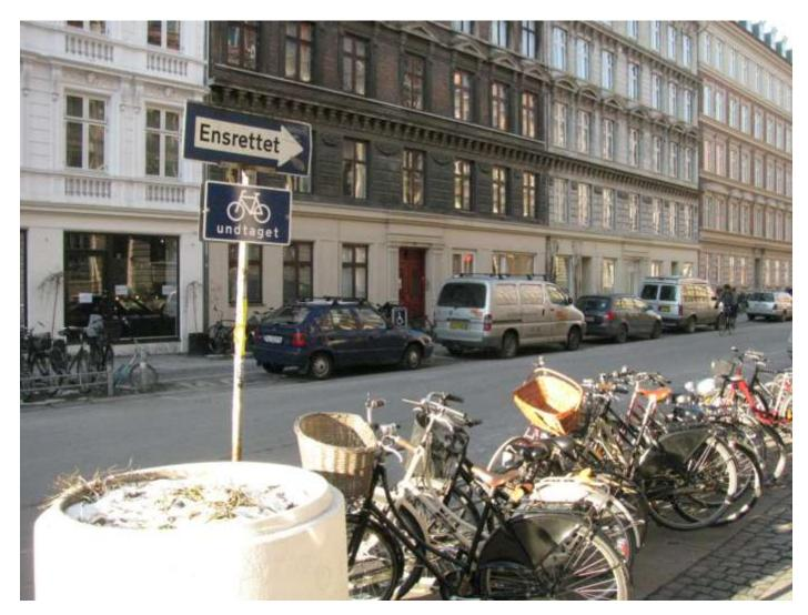
Bicycle contraflow without cycle track is marked only at intersections.
