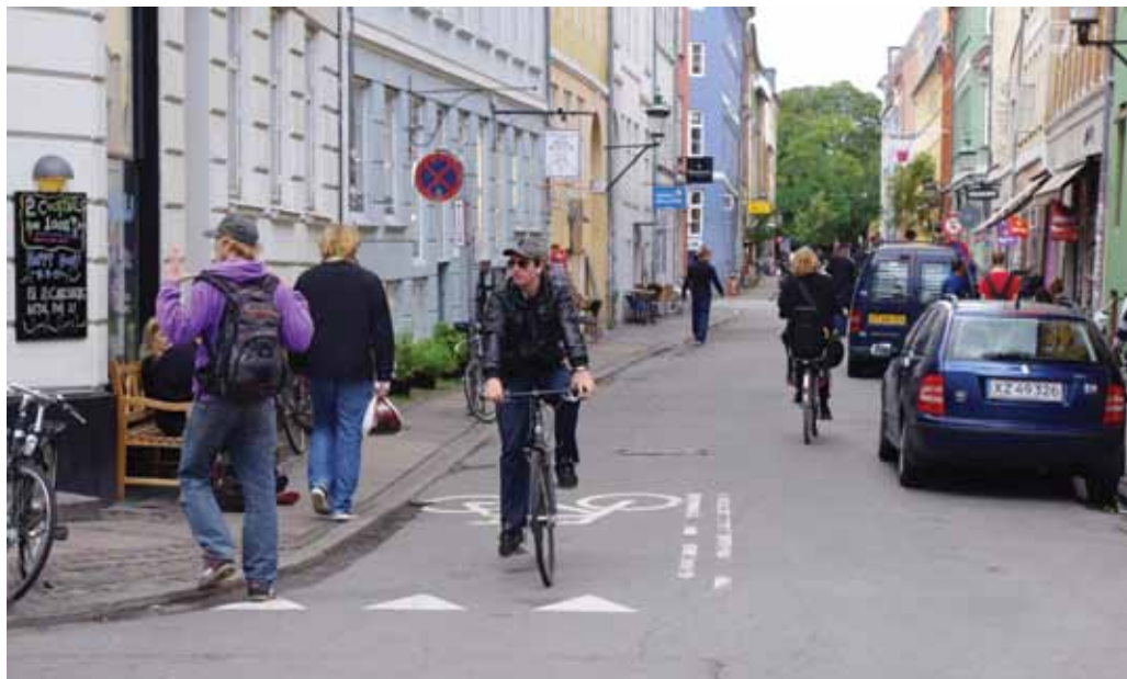
"The necktie solution" allowing contra-flow cycling on a small street in the historic centre of Copenhagen. This has the advantage that only the start and the finish need to be marked at intersections, and car parking need not be removed from the section.
