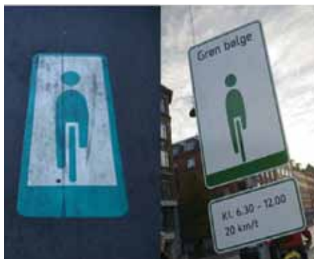
Nørrebrogade, Copenhagen. Signs and pictograms make cyclists aware of the green wave. The green wave is set for 20km/h in changing directions according to the time of day. 11.30
