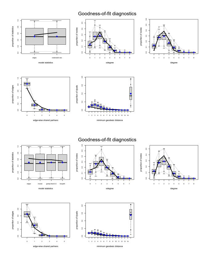
The three graphs above show the results goodness-of-fit diagnostics of Model 1, Model 2 and Model 3. It appears that in the graphs of Model 1, the black lines of empirical data are located well within the box plots of simulated data on these dimensions while it is not the case for Model 2 and Model 3. Model 1 has the best model fit.
