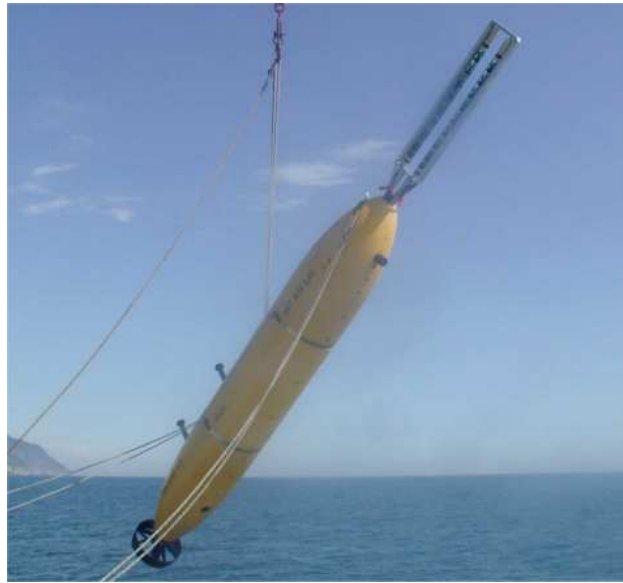
Figure 2.2: An autonomous underwater vehicle about to be launched. The large fork on the front is a sonar designed to detect buried mines. Within the hull is a transceiver which emits a “call” pulse into the water column. Beacons deployed at known locations detect this pulse and reply with a “acknowledge” pulses which are detected by the transceiver. The difference in time between “call” and “acknowledge” is proportional to the distance between vehicle and each beacon. (photo courtesy of MIT) see figure 2.2.2
