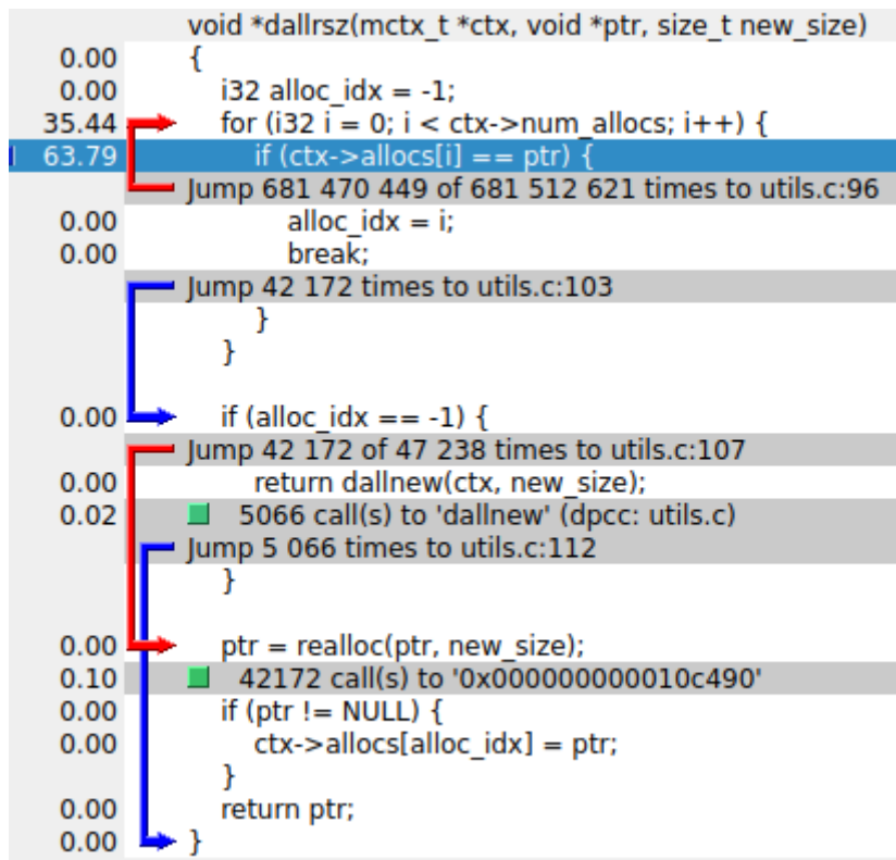
Figure 4: The linear search allocation scanning. The loop is taken tremendous amount of time for basically no useful reason.
