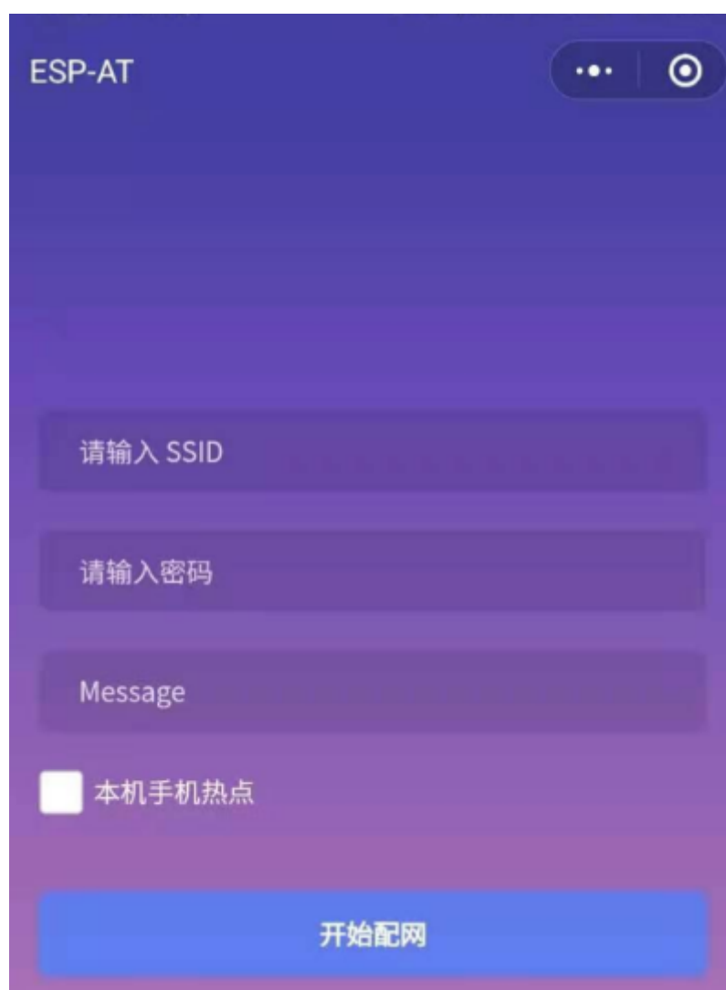
Fig. 12: Wi-Fi Provisioning Interface
