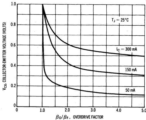
This graph shows the effect of base current on collector current. β<sub>o</sub> (current gain at the edge of saturation) is the current gain of the transistor at 1 volt, and β<sub>F</sub> (forced gain) is the ratio of I<sub>C</sub>/I<sub>B</sub> in a circuit.
