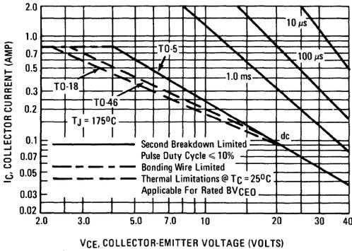
This graph shows the maximum  $I_C$ - $V_{CE}$  limits of the device both from the standpoint of thermal dissipation (at  $25^\circ C$  case temperature), and secondary breakdown. For case temperatures other than  $25^\circ C$ , the thermal dissipation curve must be modified in accordance with the derating factor in the Maximum Ratings table.
