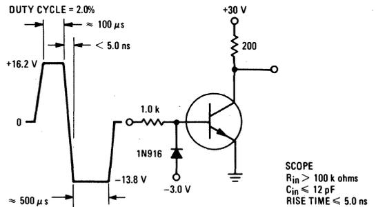
FIGURE 16 – CURRENT-GAIN-BANDWIDTH PRODUCT AND COLLECTOR-BASE TIME CONSTANT DATA
