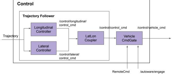
$\cdot$  In this implementation, longitudinal and lateral controls are separately calculated
