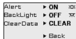
All of the accumulated value on this device, such as Dose, contact and Exp.Time can be cleared and reset to 0 manually after selecting the ClearData function.
